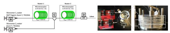
Fig. 20 Schematic representation and photographs of a continuous flow reactor for the block copolymer synthesis. The reactor system is composed of two separated syringe pumps for two tubing reactors, a micromixer tee, and a back-pressure regulator (BPR). Adapted with permission from ref. 136 (Copyright 2019 American Chemical Society).
