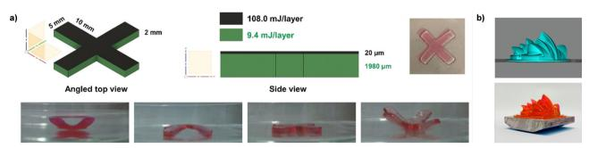
Fig. 19 (a) Synthesis of a 4D printed object capable of swelling- and desolvation-induced actuation owing to difference in mechanical properties of two layers by the spatially resolved light doses. (b) Original stl file image and 3D printed theater complex. Adapted with permission from (a) ref. 142 (Copyright 2019 John Wiley & Sons, Inc.) and (b) ref. 362 (Copyright 2021 American Chemical Society).
